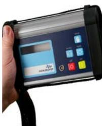
The MHC-Memo Pro is able to monitor a near unlimited number of machines on a periodic basis. In addition to storing Standard and Super Slo modes within its walk around routes, the MHC-Memo Pro can also store manually input values from any other device (e.g. a pressure gauge, kVA meter etc.). The MHC-Memo Pro can hold up to 6 routes at a time, each having up to 435 measurement points within a Site, Area, Machine & Point hierarchy.
